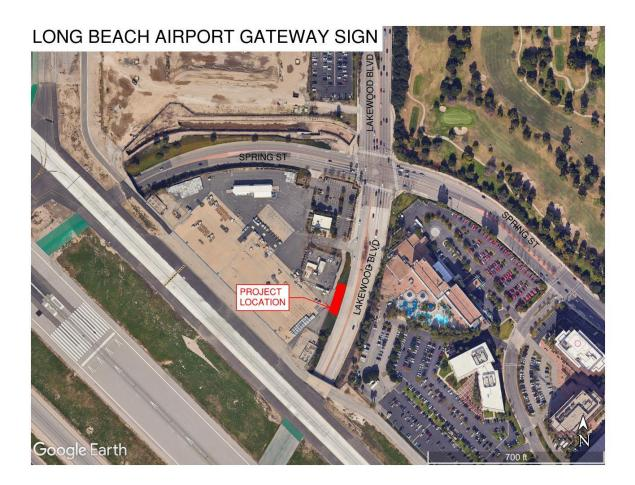
**DESCRIPTION OF WORK:** The Work to be done consists primarily of removal of existing landscaping, installation of new gateway sign approximately 12' high by 125' long near the intersection of N Lakewood and E Spring Street, installation of a concrete foundation for the sign, installation of new electrical for the lighting, new irrigation, and new landscaping.
